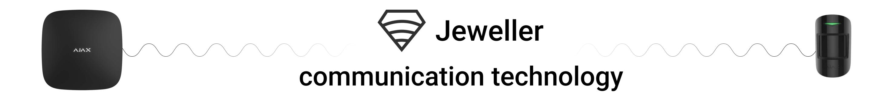
Jeweller radio protocol provides two-way communication between a hub and devices at a distance of **up to 2,000 m**. Jeweller uses time frames to synchronize communication with connected devices, authentication to eliminate forgery, and encryption to protect against data theft.
